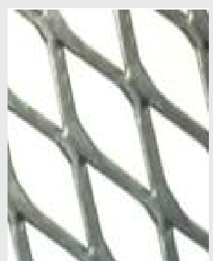
No tapering gaps that could create a trap.
